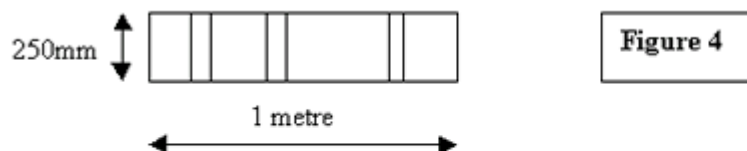
Rear panel 250 mm x 1 metre 3 off 20mm tubes cast 125mm, 500mm and 875mm from the top and 50 mm deep
