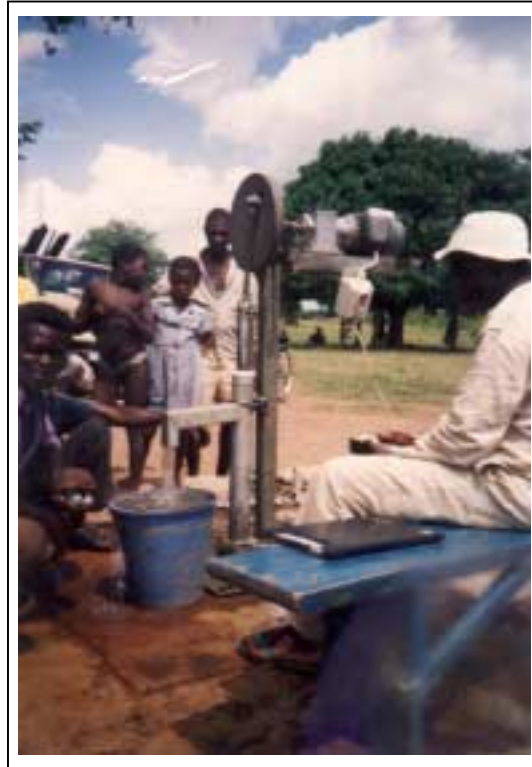
Figure 8: Test Pumping in Progress
