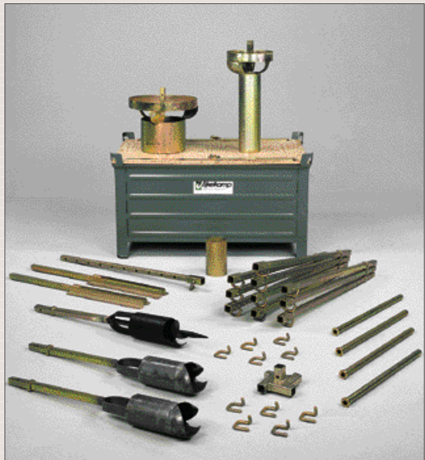
Latrine borehole drilling set
