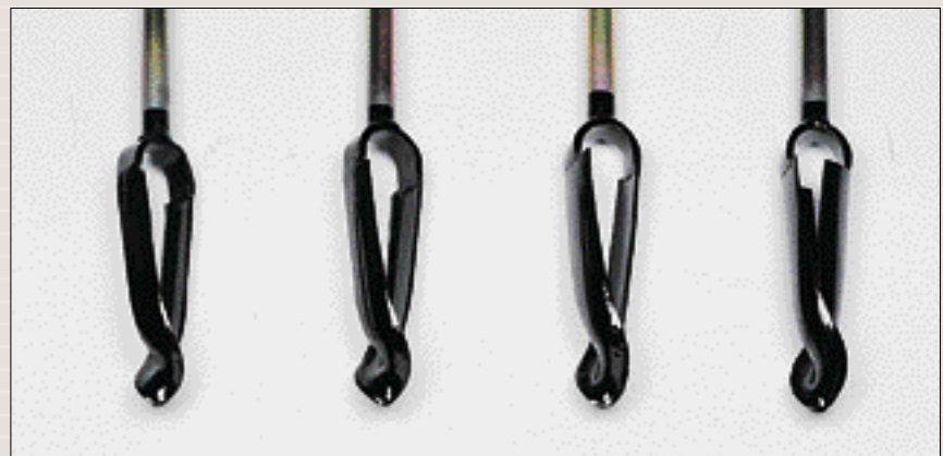
Edelman augers: clay, combination, sand and coarse sand type
