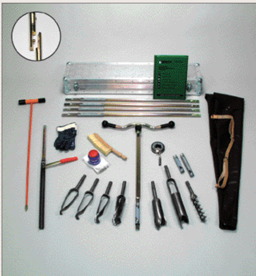
Ergonomical auger set with bayonet connection
