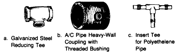
Figure 1. Service Tees Installed During Construction
