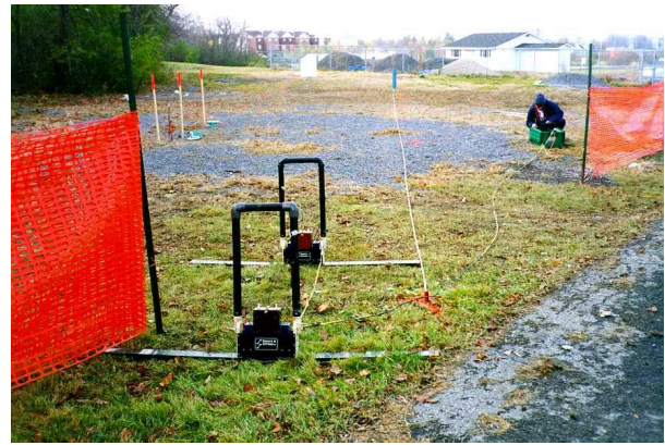
Figure 3 GPR antennas perpendicular to survey line
