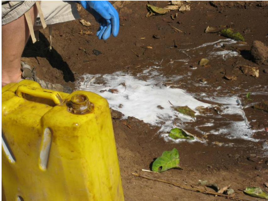
Plate 4 ~ Foaming caused by Calcium Carbonate deposition within the Jerry Can
