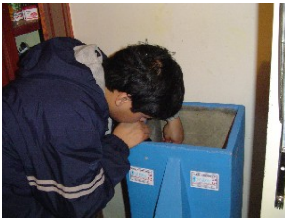
Figure 6.1: Team member Jeff Cerilles inspects the head space of a BioSand filter.
