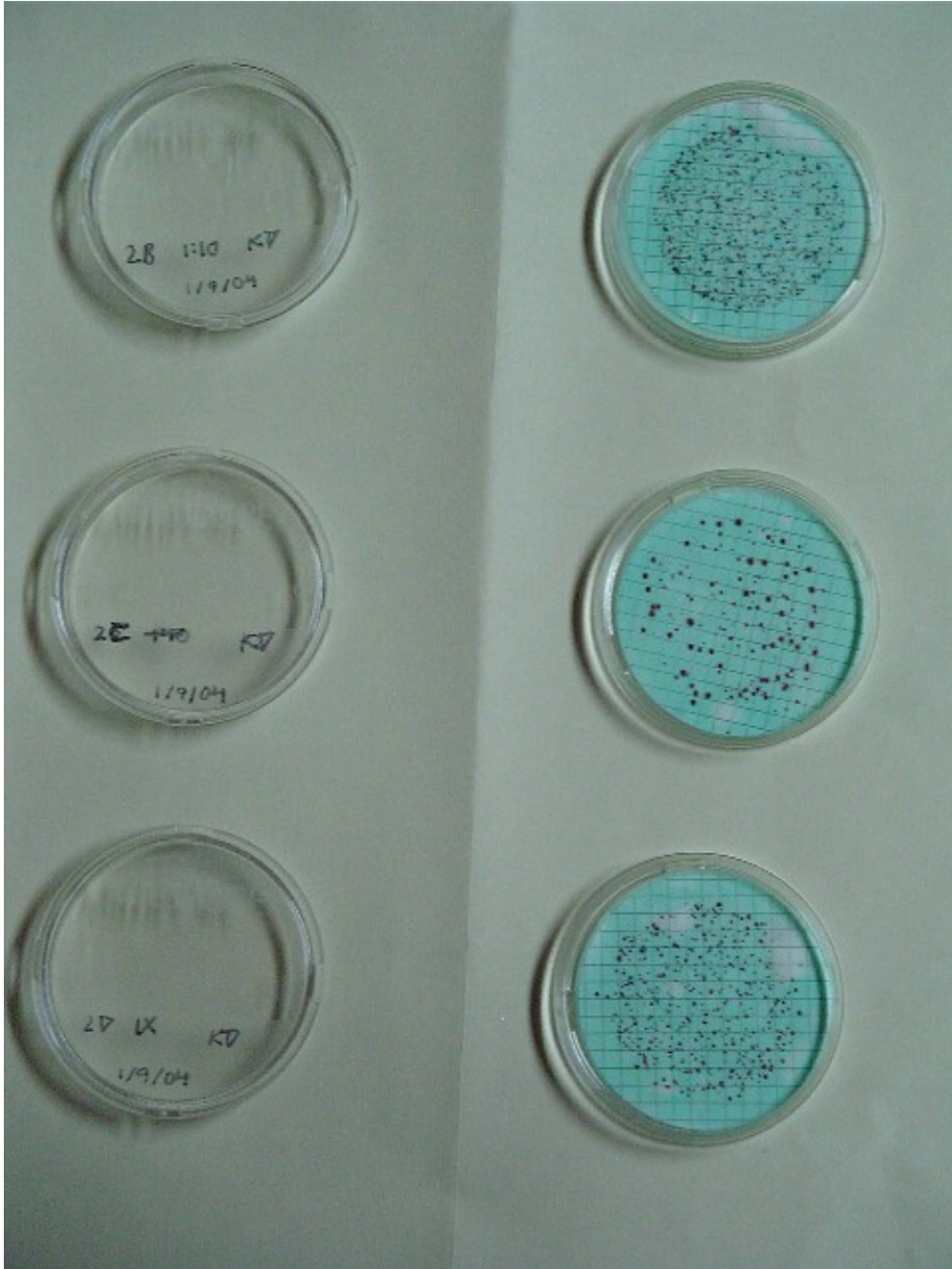
Figure 7.3: Total Coliform plates from 10 ml of source water, 100 ml of filtered water, and 100 ml of stored water in Mao, Dominican Republic, January 9, 2004.
