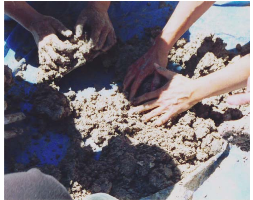
Sawdust and clay mixed with water.
