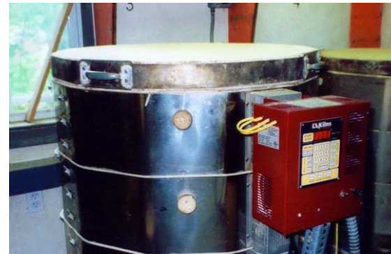
Kiln used to fire filters at SBL
